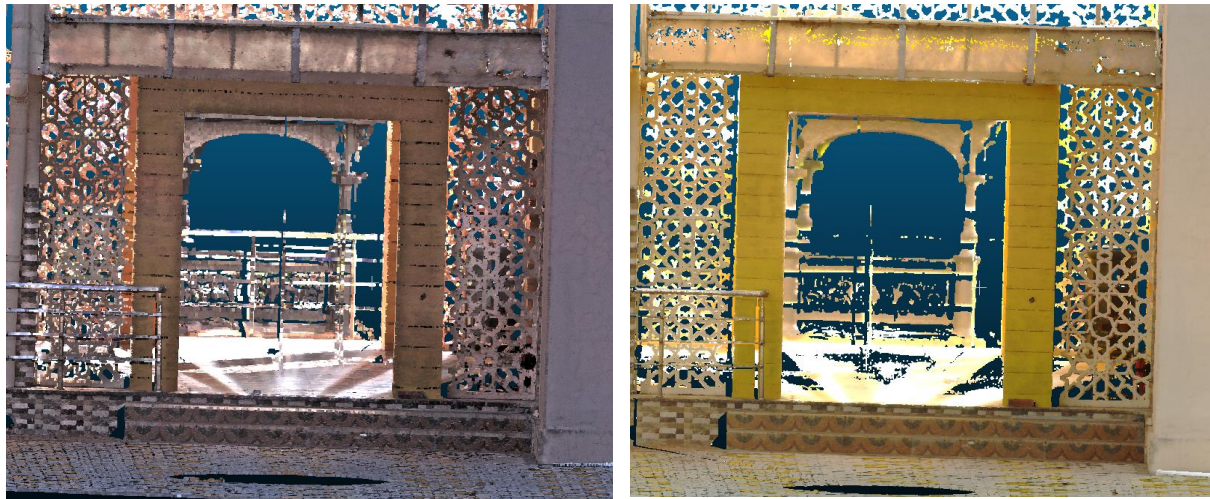
Figure 4: RGB View of point cloud data in Leica P50 scanner (left) and Faro S350 scanner (right)
