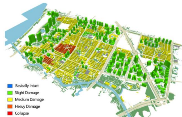
Figure 9. Various building damage state based on HAZUS Methodology using ArcGIS Software.
